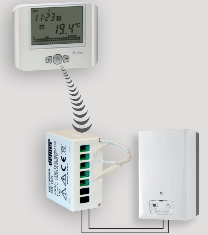
Example of connection with 1 channel remote actuator
