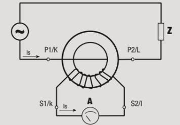
When connecting all amperometric transformers it is important to respect the directions of the current.
