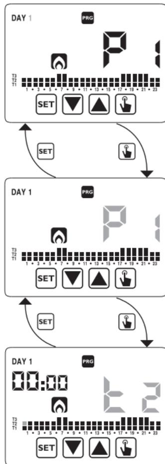
Use the keys ▲ and ▼ to change the temperature level and the key [SET] to move to the next hour. Set like this the desired level temperature for each hour of the day.
