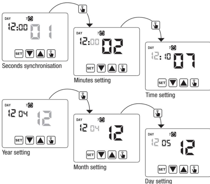
Once all values are set, press for a long time (3 seconds) the key **SET** to exit the menu of the clock synchronisation.
