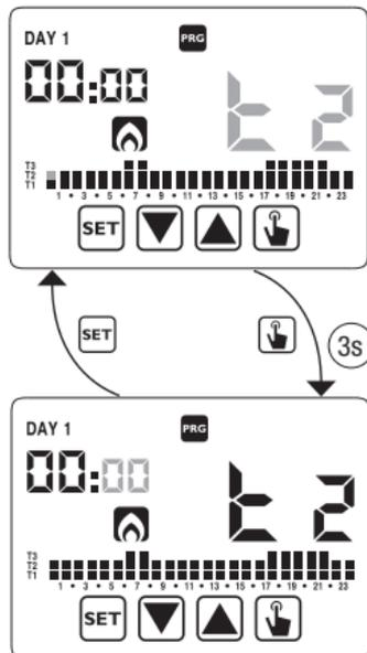
4. When the program satisfies the user's needs, go back to the days pressing twice the key [SET] and repeat for the other days of the week the operations. When all modifications have been performed, exit the programming menu pressing for a long time the key [SET].
