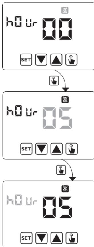
5. Once all parameters are set, to exit and to go back to the programming menu, press for a short time the key **SET**.
