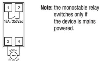
**Note:** the monostable relay switches only if the device is mains powered.
