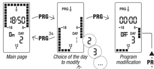
**Note:** you can exit programming even if you don't press any key within the time-out (40 seconds if the device is mains powered, 10 seconds if powered by the backup battery). The modifications are still saved.
