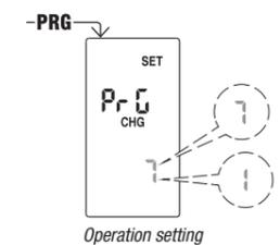
**Note:** you can exit programming even if you don't press any key within the time-out (40 seconds if the device is mains powered, 10 seconds if powered by the backup battery). In this case the modifications are not saved.
