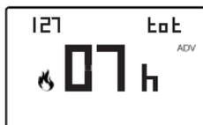
To reset the counter, keep the key
