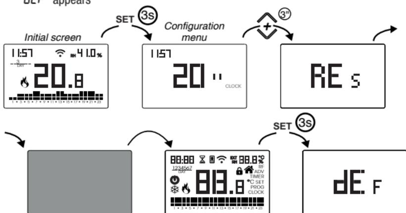
⚠ To reset if the key lock is active and you do not know the unlock password, you must remove and restore power and, when the display shows all the segments, keep the key **SET** pressed until "dEF" appears.
