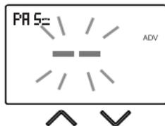
When the keypad lock is active, the symbol
