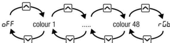
The backlighting can also be activated/deactivated from the initial screen by keeping the key
