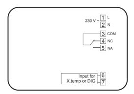
■ Thermo GSM is a wall-mounting electronic thermostat with a built-in GSM interface, available with weekly programming. The instrument performes 1B type actions and it is suitable for installations in ambient with a pollution degree of 2 and overvoltage category III (EN 60730-1).
