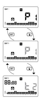
Use the keys and to change the temperature level and the key to move to the next hour. Set the desired level temperature for each hour of the day.
