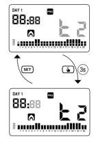
4. When the program satisfies the user's needs, go back to the day pressing twice the key (SET) and repeat the operation for the other days of the week. When all modifications have been performed, exit the programming menu pressing the key (SET) for a long time.
